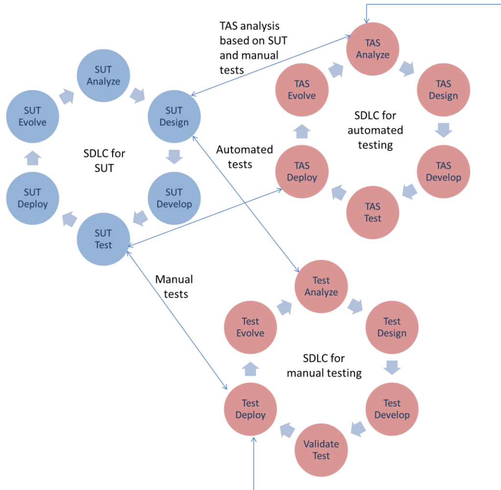
Figure 4: Synchronization example 2 of TAS and SUT development processes
